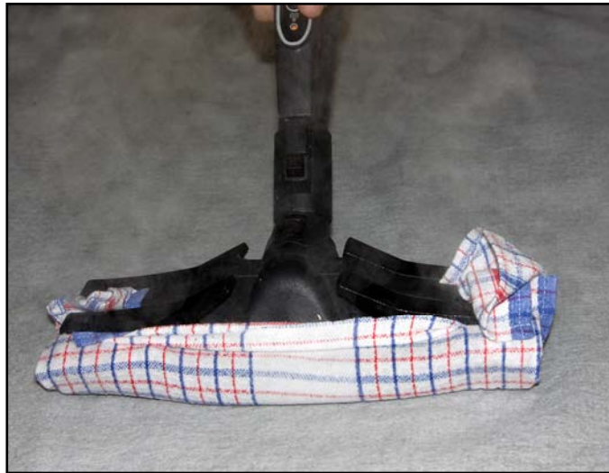
Figure 14. Covering the steam head with cloth will ensure that bugs will not be blown about, yet the temperature will be high enough to kill the insects.
